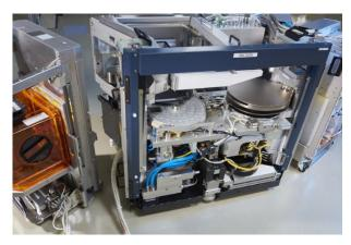
Tribological components such as bearings and guides are used under conditions beyond the limits set by suppliers: making small oscillating movements or step-scan motions under high accelerations. Vacuum environments prevent the use of conventional greases.
